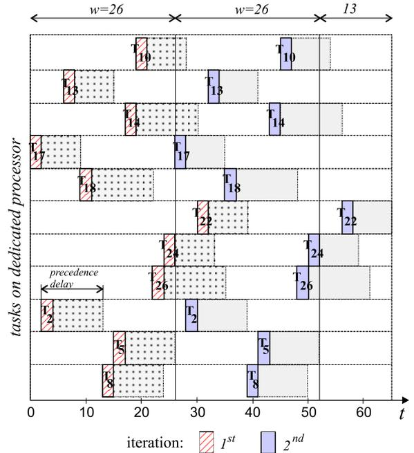
Figure 12: The schedule of the RLS filter inner loop on dedicated processor ( $w^* = w(G) = 26$ ). Each task of  $G'$  is depicted in separate line. Corresponding precedence delays represent pipelined computation and operations on other processors.
