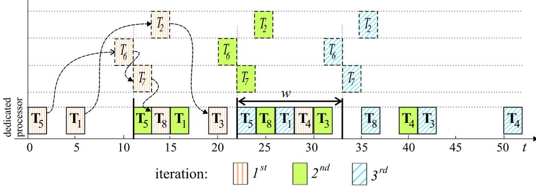
Figure 10: The schedule ( $w^* = w(G) = 11$ ) including inverse reduction to multiprocessor.
