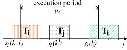
Figure 7: Processor constraint illustration example.  $T_i$  and  $T_j$  are tasks without precedence constraint ( $p_i = 3, p_j = 2$ ) with start times  $\hat{s}_i = 7$  and  $\hat{s}_j = 3$  and period  $w = 8$ .
