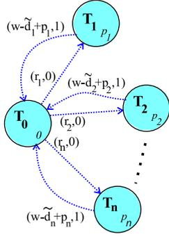
Figure 6: Polynomial reduction of Bratley's problem  $1|r_j, \tilde{d}_j|C_{max}$  to monoprocessor cyclic scheduling with precedence delays. Each independent task of the set  $\mathcal{T} = \{T_1, T_2, \dots, T_n\}$  is linked with dummy task  $T_0$  using precedence delays to specify task's release date and deadline.
