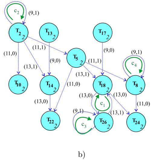
Figure 11: a) The inner loop of RLS filter. Constant  $N$  determines the filter order. b) Corresponding reduced graph  $G'$  contains four circuits  $c_1, c_2, c_3$  and  $c_4$  with critical circuit  $c_1$  since  $w = \max\{26/1, 9/1, 9/1, 9/1\} = 26$ .
