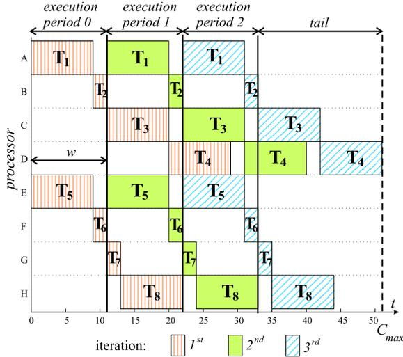
Figure 4: A feasible periodic schedule ( $w = 11$ ) optimal with respect to minimal  $w$ .
