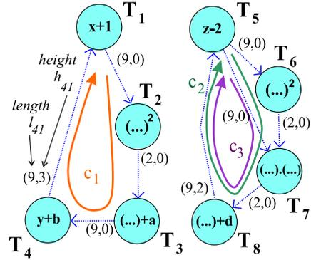
Figure 3: An data dependency graph  $G$ , representing operations and data of the computation loop in Figure 2. Operation power three is realized as power two and multiplication. The  $G$  contains three cycles  $c_1$ ,  $c_2$  and  $c_3$  with average cycles times  $\{29/3, 22/2, 20/2\}$ . With respect to the critical circuit is  $c_2$  with  $w = 11$ .
