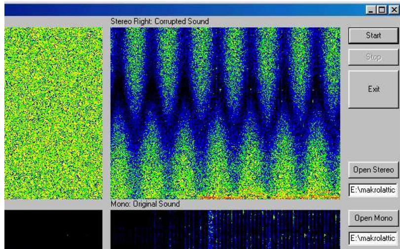
Figure 13: Spectral analysis of input and output signals of the optimized RLS filter.
