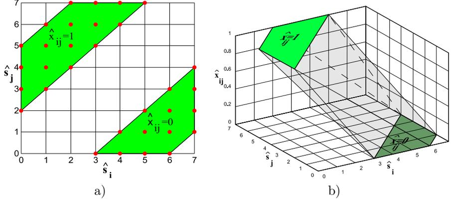
Figure 8: State space of feasible schedules given by Double–Inequality (12) of the example from Figure 7. a) State space of feasible start times  $\hat{s}_i, \hat{s}_j$ . b) Equivalent convex continuous state space.
