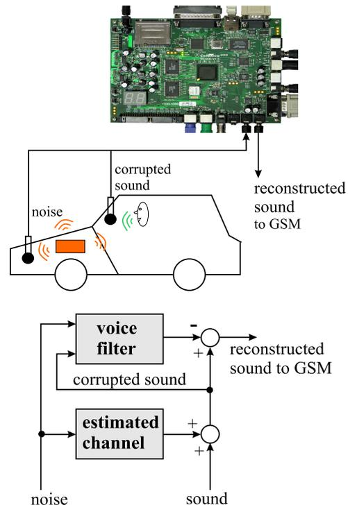
Figure 1: An illustration of active noise cancellation – an adaptive RLS filter estimates parameters of changing channel in order to reconstruct original clear sound.
