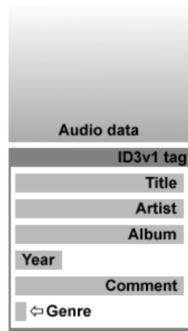
Figure 4: Internal layout of an ID3v1 tagged file[27].
