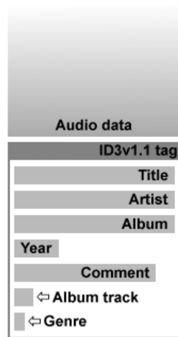
Figure 5: Internal layout of an ID3v1.1 tagged file[27].
