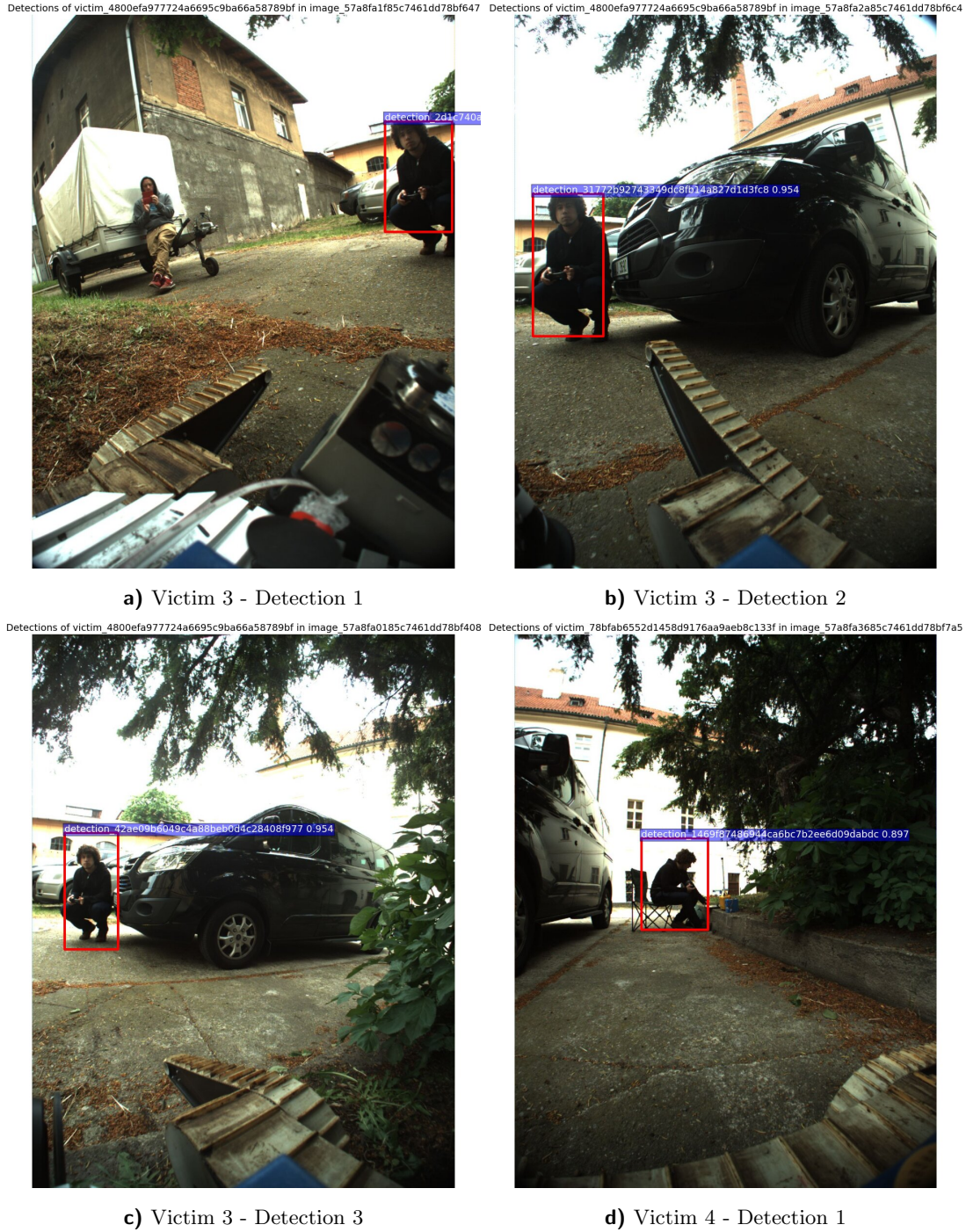
Figure 5.2 Resulting "victims" for test scenario 1 part 2 (see 5.1.1). Figure a), b) and c) depict Victim 3 whereas d) shows victim 4. Notice that Victim 3 in a) is detected in a different camera frames than in b). Detection boxes are marked red.
