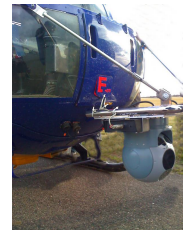
(b) The inertially stabilized airborne camera platform attached to a helicopter has to withstand significant vibrations caused by the carrier.
