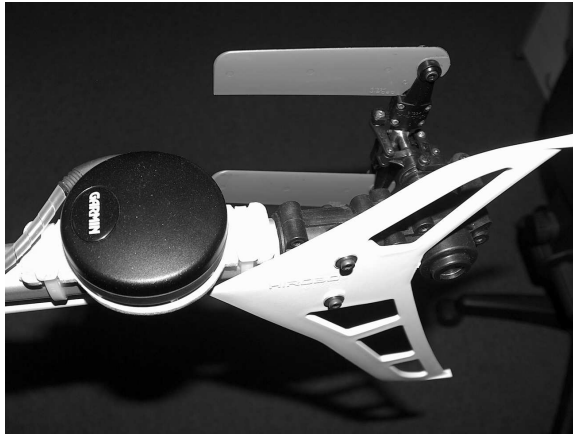
Figure 3.4: GPS receiver, mounted on the tail of the UAV
