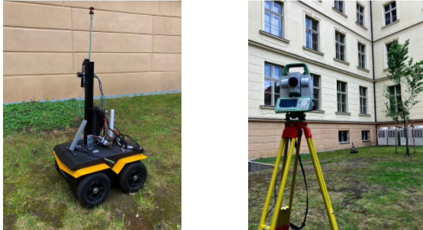
Figure 5.1: Jackal platform with camera (on the left), lidar and a prism for tracking its position by Leica Total Station during traversal of a path (on the right). All evaluated vt&r system's were deployed on the Jackal platform.
