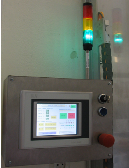
Figure 8.1: Operating panel with door lock, reset button, and emergency stop button.
