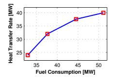
Figure 3.3: Fuel consumption characteristics of the boiler B1
