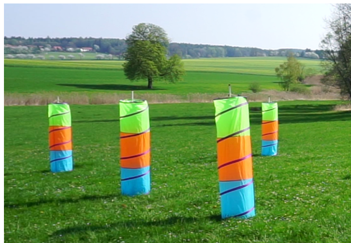
Figure 28: A simulated forest used for the experiments. The models of the trees are formed by a playground crawling tunnel secured on a metal pole.
