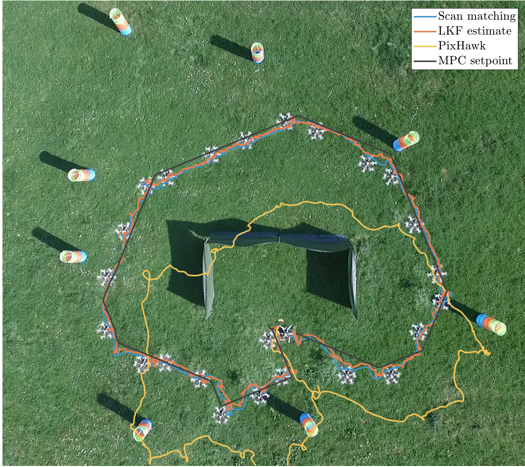
Figure 37: A top down view of the experiment. The image is stitched from a video with the UAV position snapshot taken every 10 seconds. The overlay shows, that the position estimates match the actual flight trajectory.
