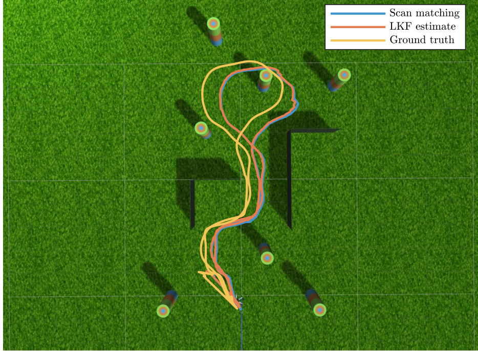
Figure 25: An aerial view of the flight area in the simulator. The UAV is hovering at the initial position of the trajectory \mathbf{x}_0 . The largest error around 0.5 m occurred in the top of the map due to low number of points in laser scans.
