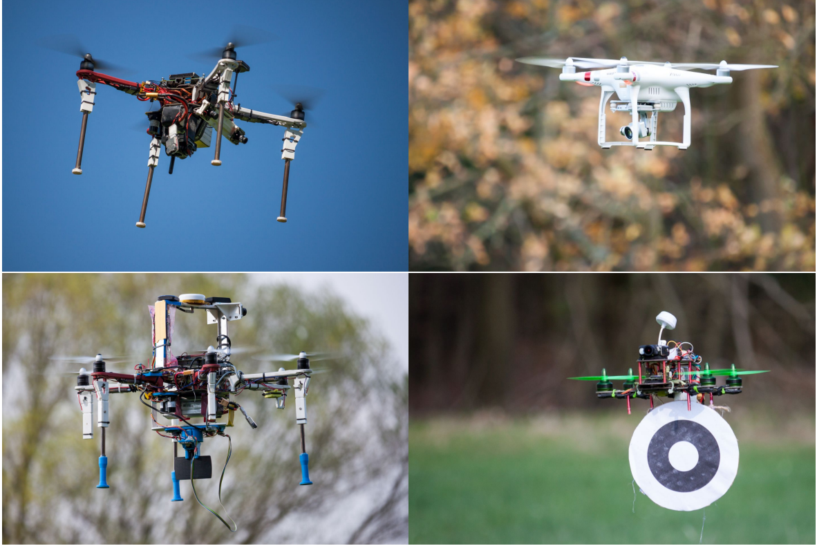
Figure 1: Examples of different UAV types. The photo at the top left corner shows a custom built UAV on the DJI F450 frame. The commercially available DJI Phantom 3 Professional is in the top right corner. The bottom left corner shows the DJI F550 frame equipped with hardware for RFID signal detection. In the bottom right corner is a photo of A250 racing drone frame equipped with WhyCon localization marker.
