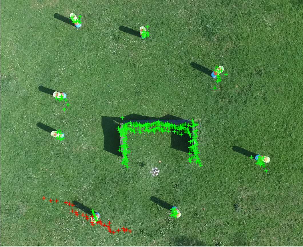
Figure 31: An aerial view of the experiment conducted for mapping module verification. The final map obtained after the whole experiment is visualized by crosses representing the global point cloud. The green color is used for correct points while outliers which should not be present are depicted by red. Some of the points do not seem to be perfectly aligned to the obstacles which is not an error of mapping but a result of the lens and perspective distortion.
