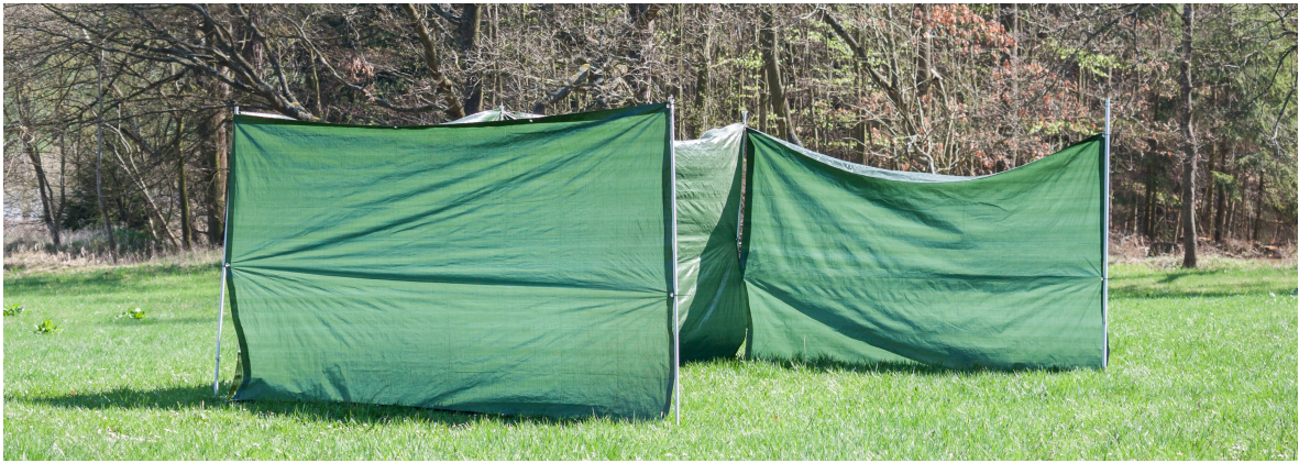
Figure 27: A model of a U-shaped room built from garden sails. The purpose of the room is to simulate localization in a typical indoor environment.
