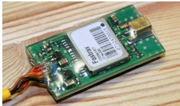
Obr. 3.9: DPS s GPS modulem iTrax03-s
