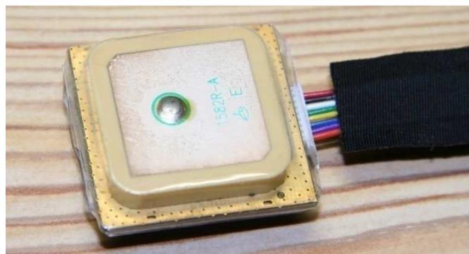
Obr. 3.12: GPS modul EB85A
