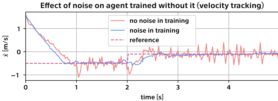
Figure 4.12: In the case of velocity tracking, training with noise makes a notable difference when noise is present.
