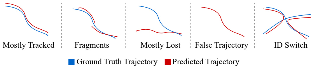
Figure 2.1: Visualization of the classical MOT metrics. Blue denotes the ground-truth trajectory and red the predicted ones (adapted from [26]). (for the final figure false alarm will be left out and all cases will be separated by vertical lines)
