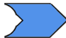
Figure 24 - Function block that can have both analog and logic input (generic left side)
