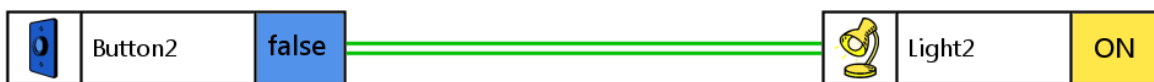
Figure 34 - On/off light controlled by a touch button – Implicit definition, compare with Figure 36
