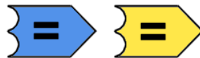
Figure 7 - Color distinguishes which comparator results in false (blue) and which true (yellow)
