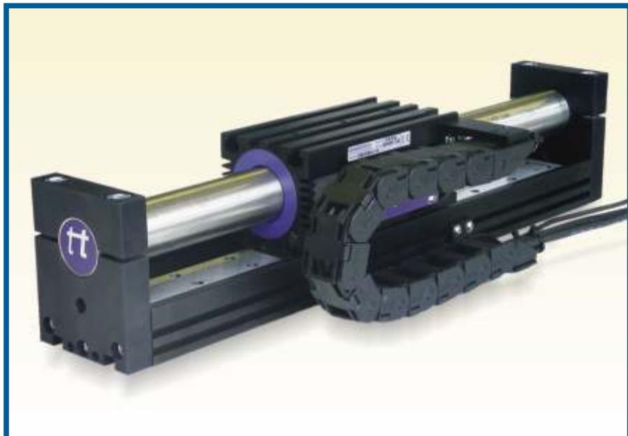
ThrustTube Module products comprise the patented ThrustTube motor components mounted in a robust extruded aluminium channel to make a ready-to-use motion axis. The motors are electrically identical to standard brushless drives and can be powered by a range of conventional servo drives.
