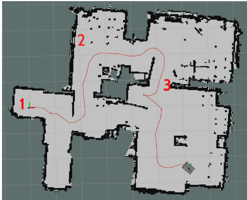
Figure 5.4: Experiment 1: Final map created in autonomous mode. Executed path is red.
