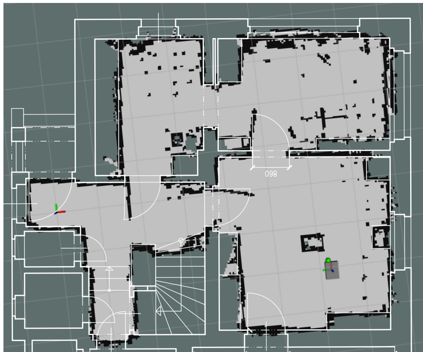
Figure 5.5: Experiment 1: Comparison of the created map and construction plan.
