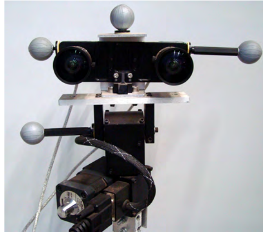
(b) Stereo cameras of ExoMader with retro-reflective balls
