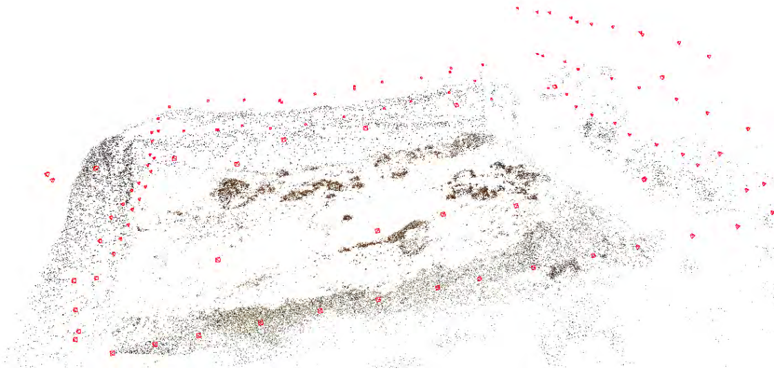
Figure 5.6: Camera positions and orientation of the 113 images taken around the testbed
