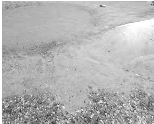
(c) Simulated terrain by means of laser scan and high resolution image projection
