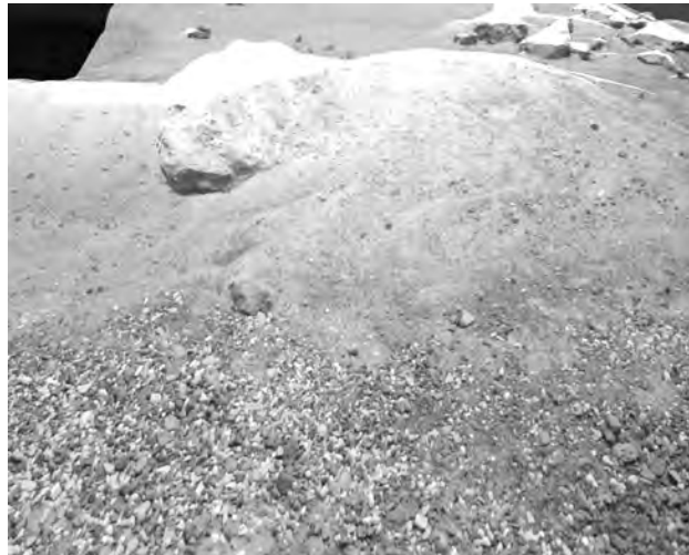
(i) Simulated terrain by means of laser scan and high resolution image projection
