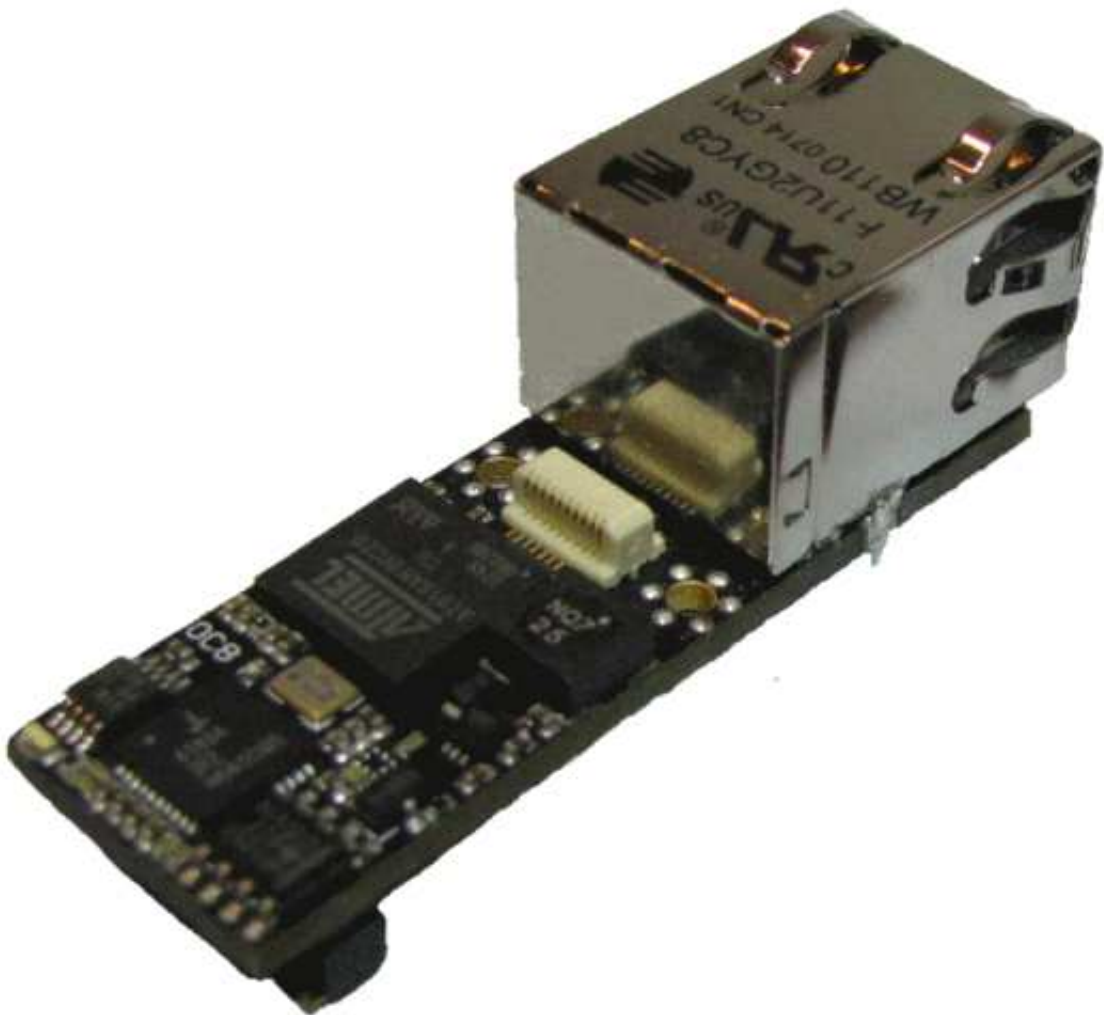
Figure 3.2: The embedded processor module Linux systems OC8-S
